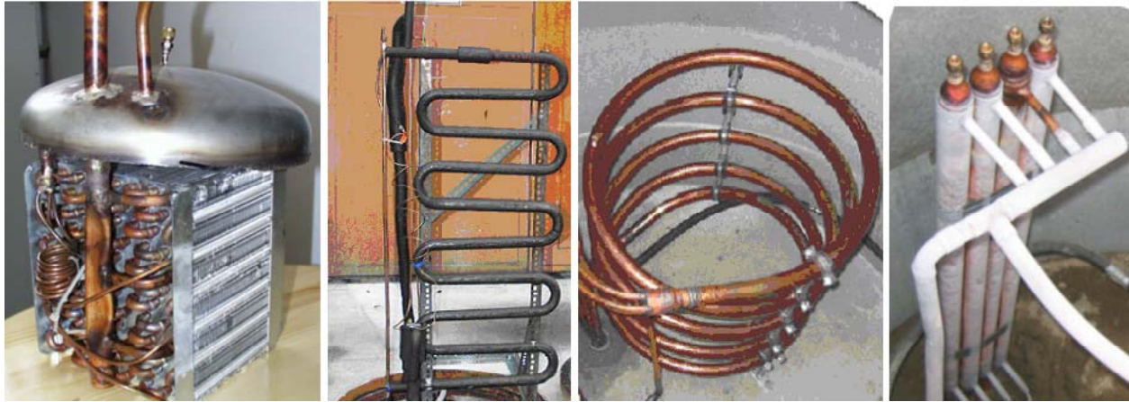
Fig. 6. Different probe head geometries (pot, serpentine, spiral, and vertical type)
