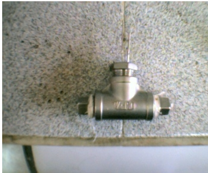
Fig. 4. On-line monitoring electrochemical sensor.
